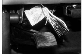
26. Connect the Muncie Blue/ White wire to the Ford Blue / White wire; circuit PTO-RELAY.
